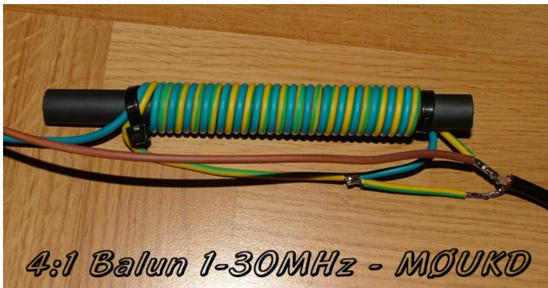
4:1 Voltage Balun used on Carolina Windom Antenna's
